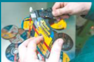
Visual control of all geometric dimensions of the wheel;
