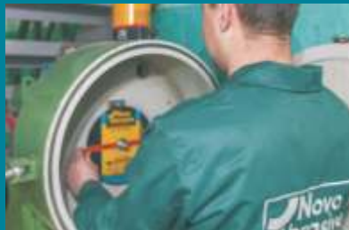
Safety test – wheel bursting speed test
