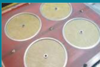
Placing of the second reinforcing element
