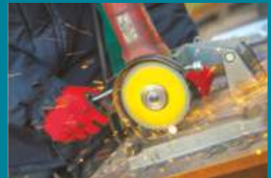
Cutting test – a test for wheel durability
